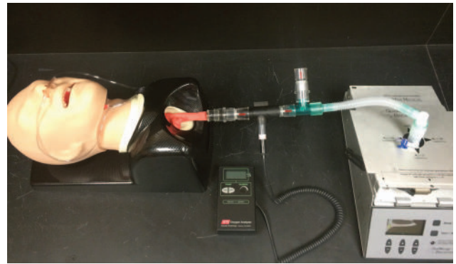
Fig. 1. Adult model with test lung and polarographic oxygen analyzer.
